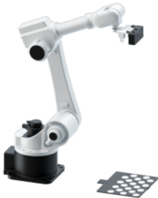
Hand-Eye Calibration in the EIH Setup (Multiple Random Calibration Board Poses)
