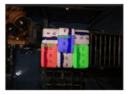
• The dimensions input in the **Recognize Center Poses of Sacks** Procedure differed greatly from recognized ones. Thus, the dimensions of the sacks could not be verified, and no output was obtained from Mech-Vision.
