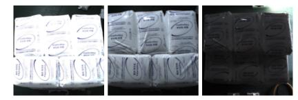
• The adjusted white balance was not appropriate for the capture of 2D images. As shown below, the image on the left was captured under incorrect white balance, while the image on the right was captured under correct white balance.
