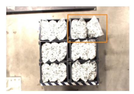
• There was severe deformation in the turnover box, or a large difference in the size of the turnover box, which was significantly different from the point cloud model, resulting in a low turnover box pose score from 3D matching and no output from the Mech-Vision project.
