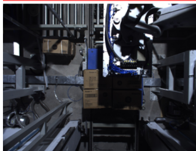
Bad example: occluded by the robot arm.
