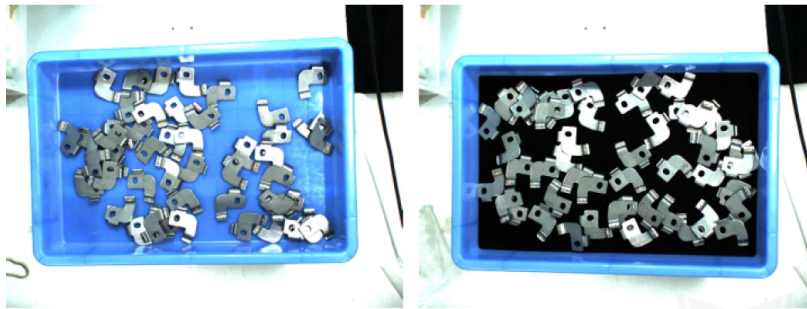
Bad example: The background in the training data (left) is different from the background in the actual application (right).
