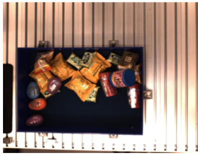
Color distortion can be avoided by adjusting the white balance.
