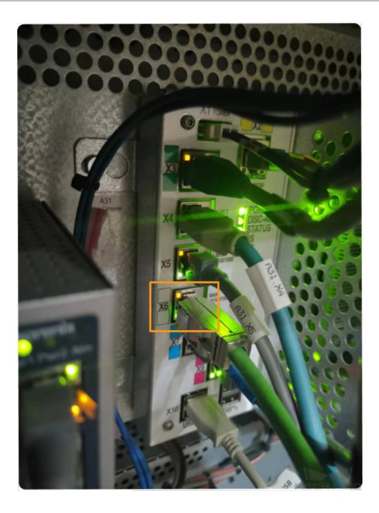
**Hint:** If you only need to load the master-control program via RobotStudio, you can use either LAN port or WAN port to connect the robot controller. However, in order to enable visual communication, the Ethernet cable can only be connected to the WAN port.
