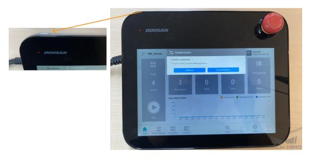
3. On the home screen of the teach pendant, press **Setting** in the bottom panel, and then press **Robot Update** to confirm whether the firmware, which is GV02080000 in the figure below, version is V2.8.
