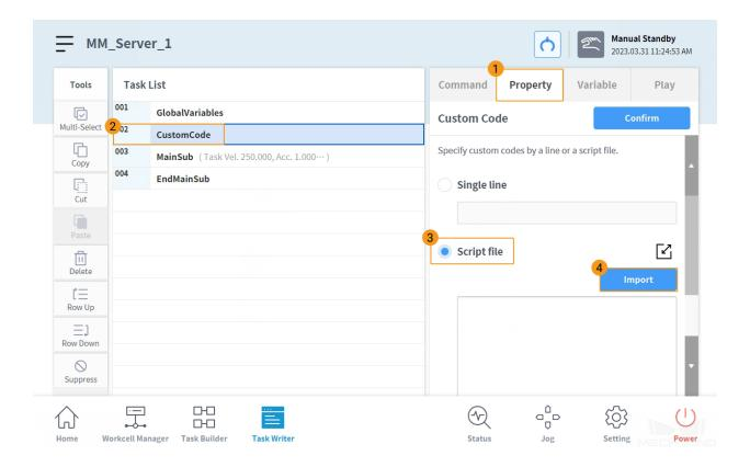
4. In the pop-up window, locate and select the MM\_Server.txt file, and press OK at the end.
