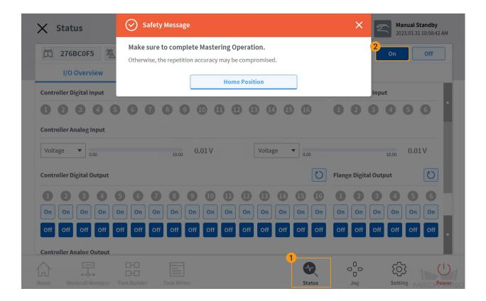
5. Press and hold the **Home Position** button until an **Information Message** window pops up. The pop-up window will disappear after a few seconds, which indicates that the robot has moved to the home position. Then press the exit button to close the **Safety Message** window.
