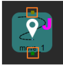
Figure 7 Input and output port of module
