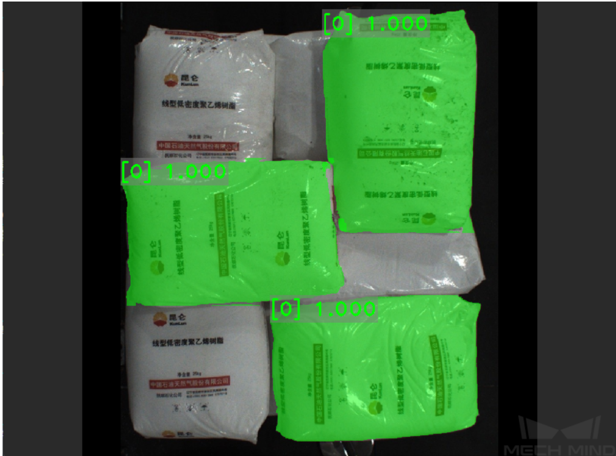
Figure 3. A sample result of Instance Segmentation (Color Image)
