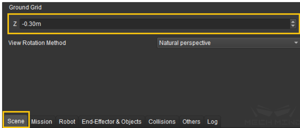
Figure 25 Adjust the Ground Height in Mech-Viz Finally, the point cloud of the calibration board will be displayed as shown in Figure 26 .
