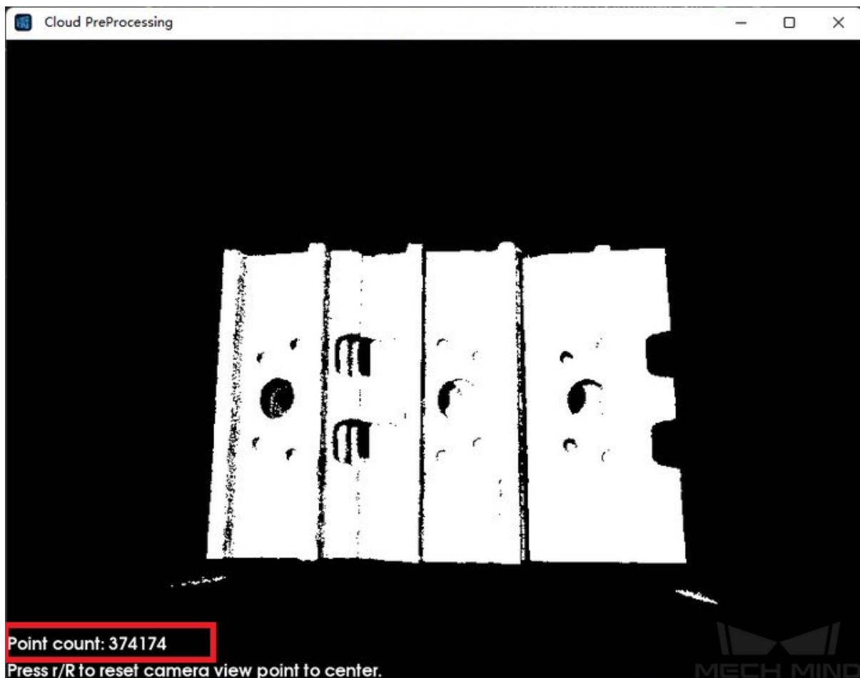
Figure 4. Point count of a point cloud
