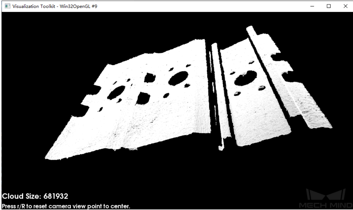
Figure6 Input Point Cloud Image to be Matched.
