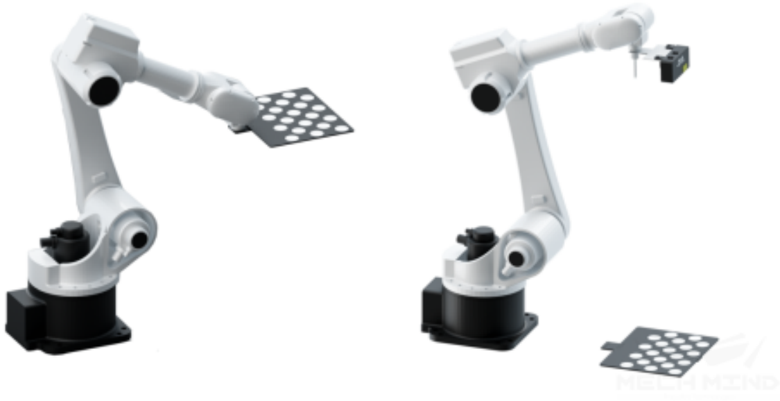
Figure 1. Installation/Placement of the calibration board
