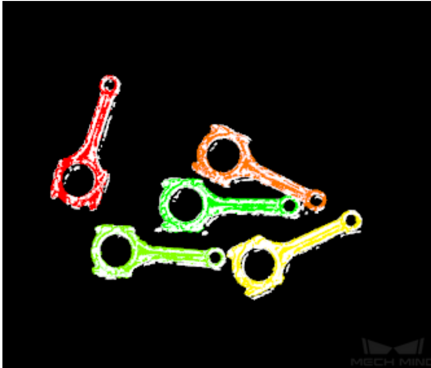
Figure 7. A sample result of 3D Matching
