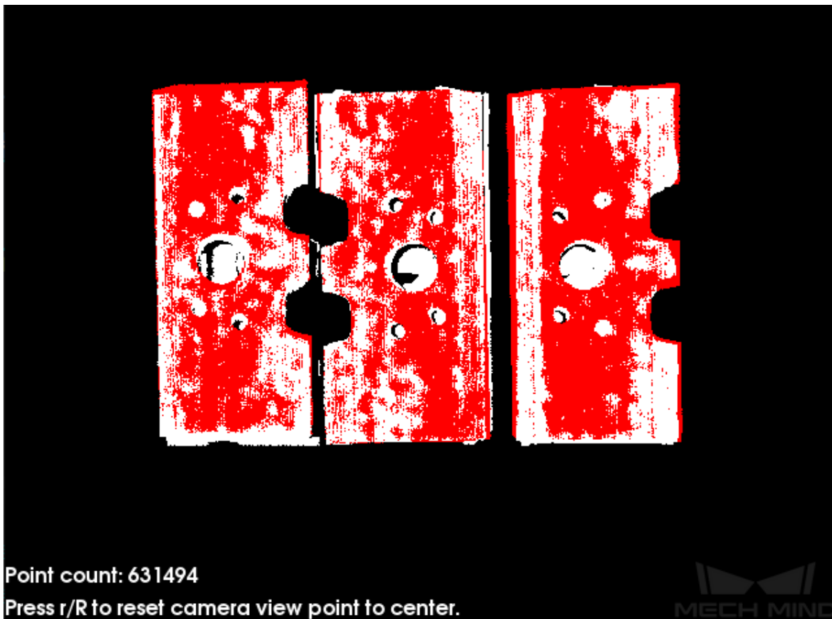
Figure 2 Multi-Template 3D Fine Matching Output
