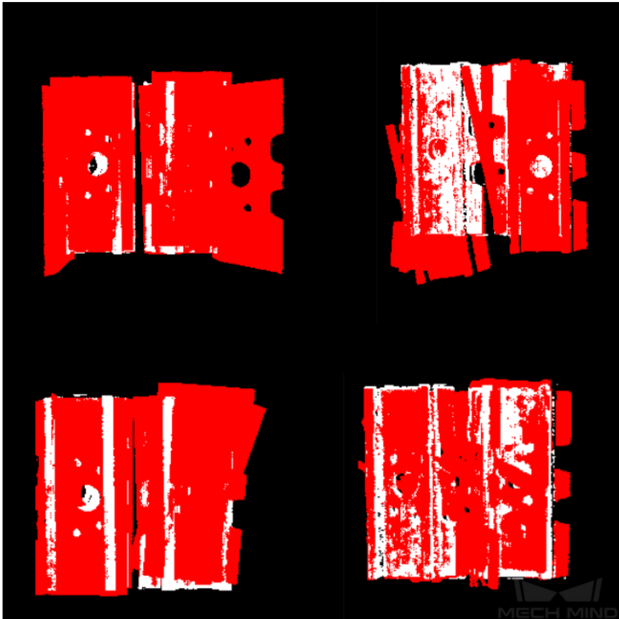
Figure 6 Comparison of Sample Interval Parameter Adjustment Results of Model Point Cloud
