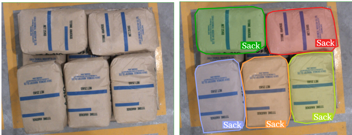
Figure 3. Segmenting sacks in an image in a palletizing/depalletizing project
