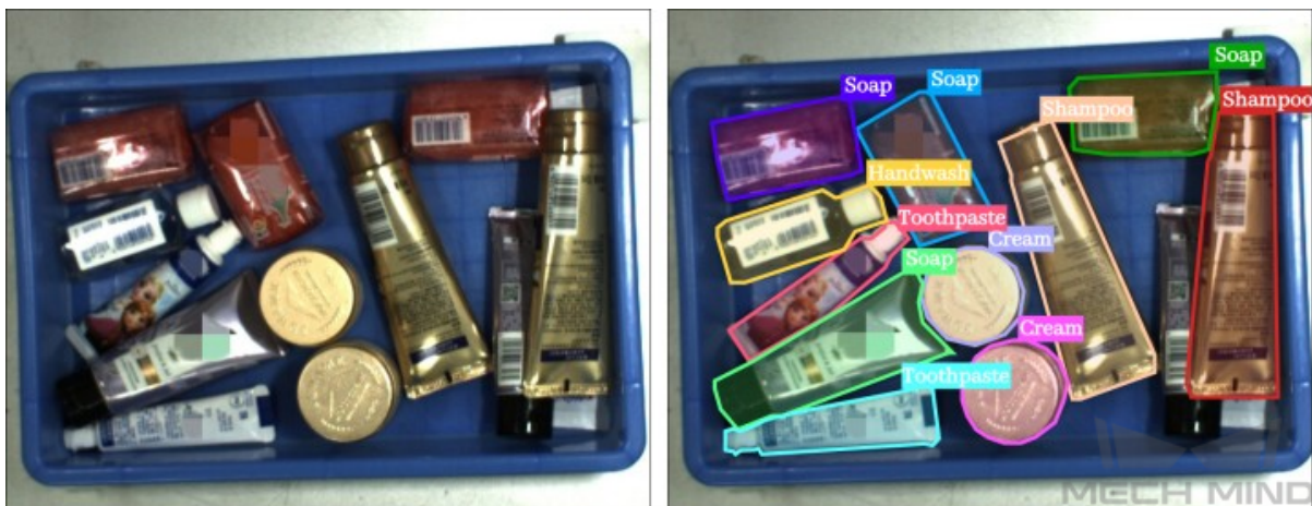
Figure 5. Segmenting goods in an image in an order picking project
