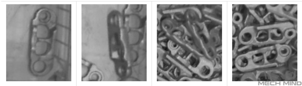
Figure 10. Lying flat, standing on sides, overlapping, and parallelly placed
